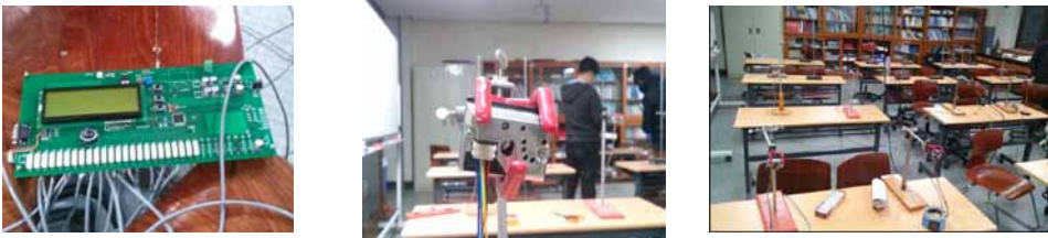
[Fig. 20] Setting for measuring concentration of fine dust
