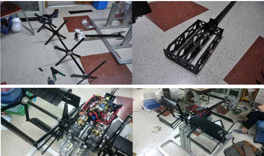
[Fig. 26] Blade hub(upper left), main frame(upper right), motor and electrical device(lower left) assembled 2-rotor cycloidal system with variable camber airfoil(lower right)
