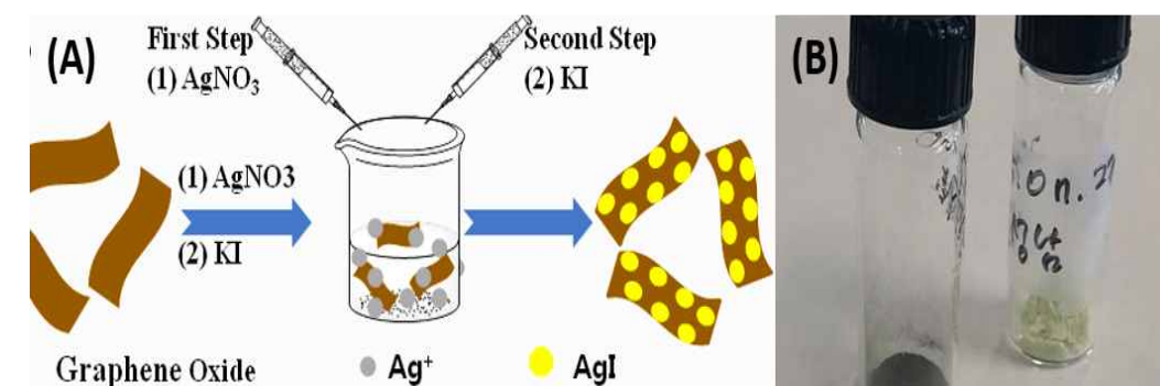
[Fig. 2] (A) The way to compose AgI-RGO nanocomposites (B) AgI, AgI-RGO nanocomposites
