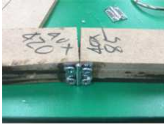
[Fig. 20] Links using hinges
