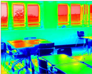
[Fig. 18] Measuring luminance(1st Mock up)
