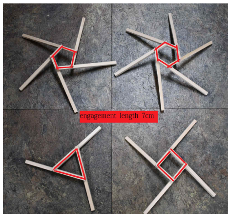
[Fig. 19] 3, 4, 5, 6-nexorades with constant Engagement lengths(7cm)
