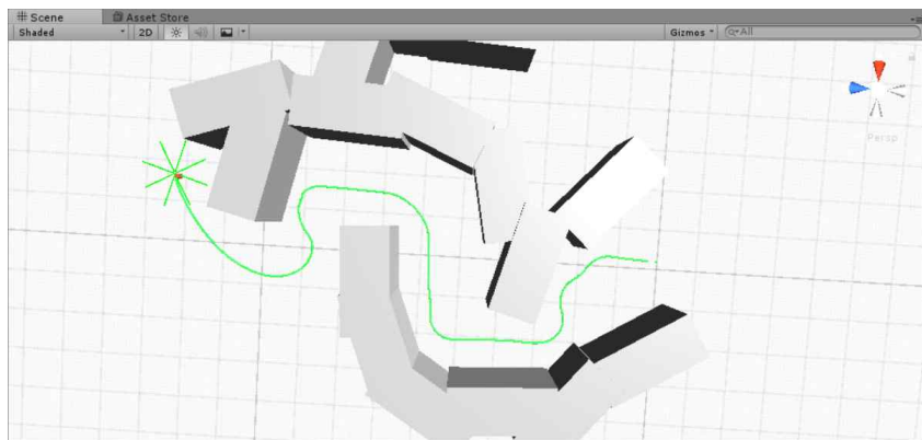
[Fig. 11] Final result for the simulation of obstacle avoidance algorithm
