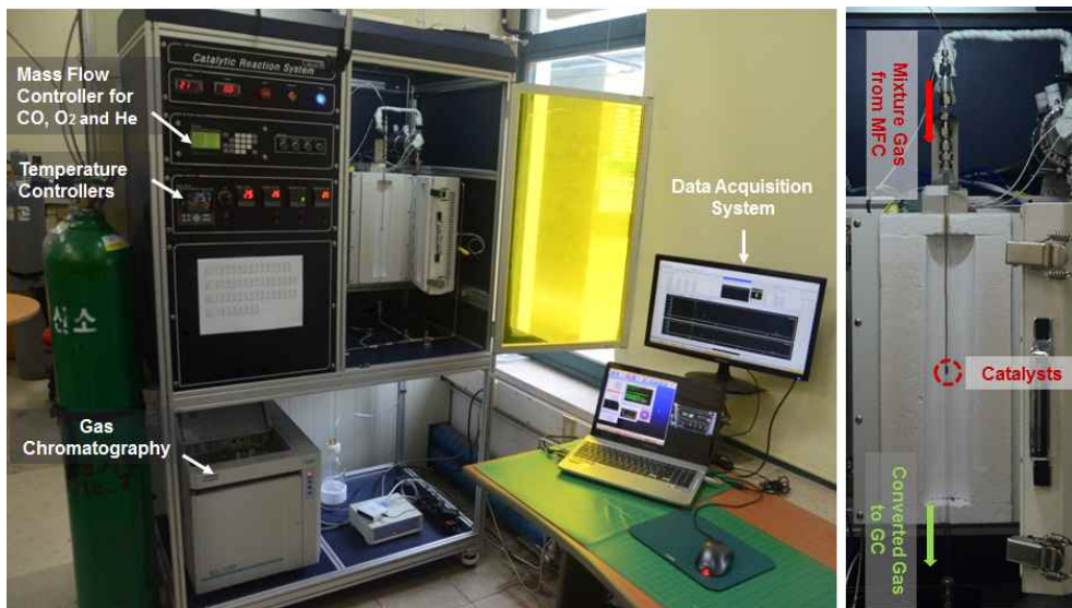
[Fig. 10] Reactor and Gas Chromatography(GC) for analysis of carbon monoxide oxidation method
