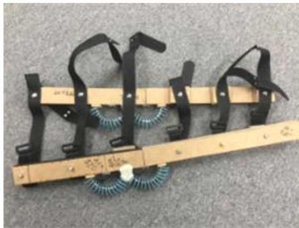
[Fig. 21] Completed exoskeleton assist device
