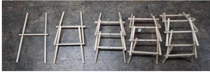
[Fig. 8] Five types of Da Vinci bridges with constant total length
