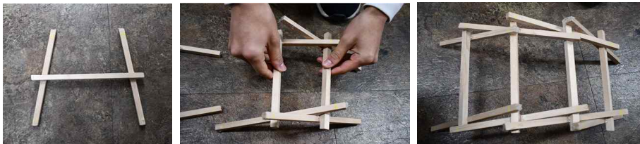
[Fig. 7] Procedures making the Da Vinci bridge. The left picture shows a unit structure.
