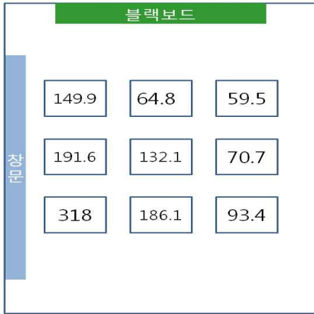
[Fig. 7] Desk surface illumination by Simulation
