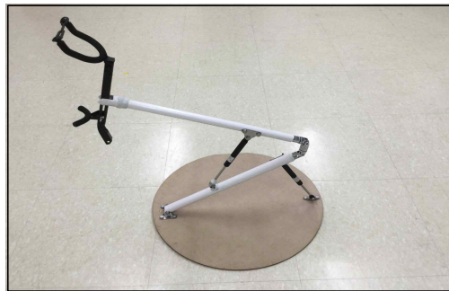
[Fig. 9] Completed vertical piston type manipulator
