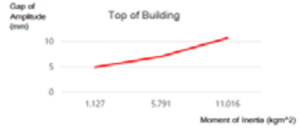
[Fig. 18] The amplitude of first vibration depend on moment of inertia, when the disk is attached to the top of the building.
