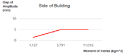
[Fig. 17] The amplitude of first vibration depend on moment of inertia, when the disk is attached to the side of the building.
