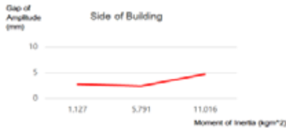
[Fig. 21] The amplitude of third vibration depend on moment of inertia, when the disk is attached to the side of the building.
