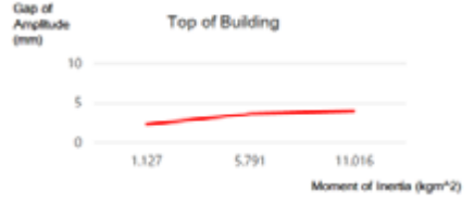
[Fig. 20] The amplitude of second vibration depend on moment of inertia, when the disk is attached to the top of the building.
