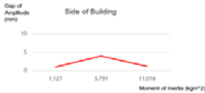
[Fig. 19] The amplitude of second vibration depend on moment of inertia, when the disk is attached to the side of the building.
